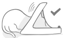
When a pet places its head into the hoop on the front of the feeder, the microchip reader is activated.
